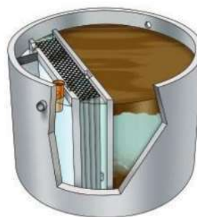
Figure 25 : Micro station à culture fixée (EPUR®)
